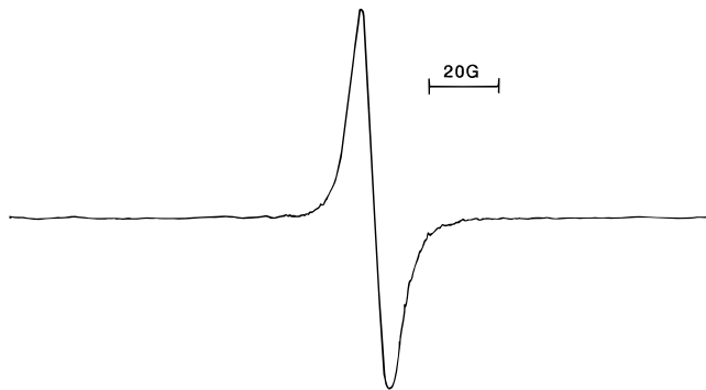
Figure 5. X-band EPR spectrum of the 8-oxodG radical anion generated by \gamma -irradiation in a 10 M LiCl glass at 77 K and annealing to 155 K to remove the background solvent signals. In contrast to the guanine radical anion the 8-oxodG radical anion does not C-8 protonate on annealing.
